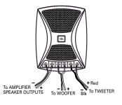
Figure 8B. Locating wiring connections on the GT0506c woofer. Other woofers are wired similarly.
